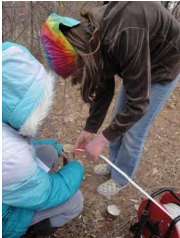
BEMP students measuring depth to groundwater
